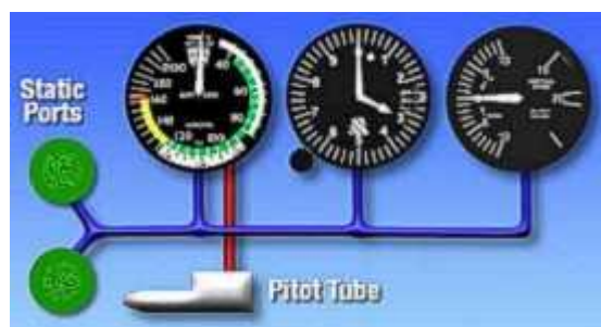
Figure 1, pitot/static system schematic. Click image for larger version.
